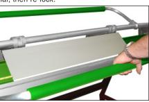
C. Rotate front hinge up to flatten angle against F-Bar to complete hem. Note: It is recommended that you make practice bends with scrap until satisfied with results.
