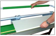
B. Place material against F-Bar with angle of material just bent set between Stainless edge and front hinge.
