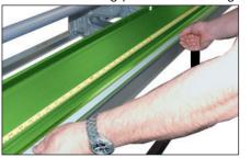
A. Insert material into brake to your measurements and lock brake. Bend flat against stainless strip. Unlock brake, remove material, then re-lock.
